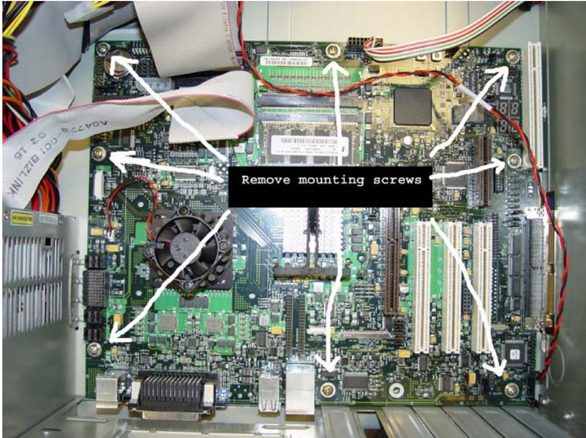
4. Make sure any other wires connected to the motherboard are disconnected.
