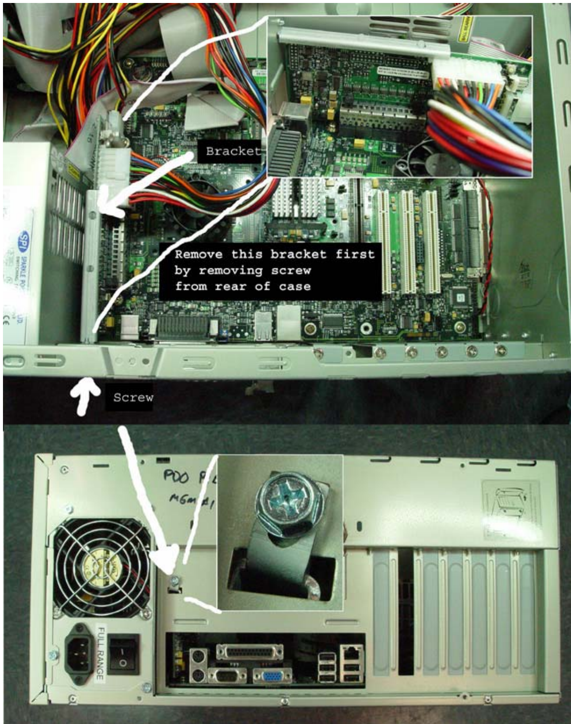
Figure 11. Removing the Screw and Bracket From the Chassis Back
