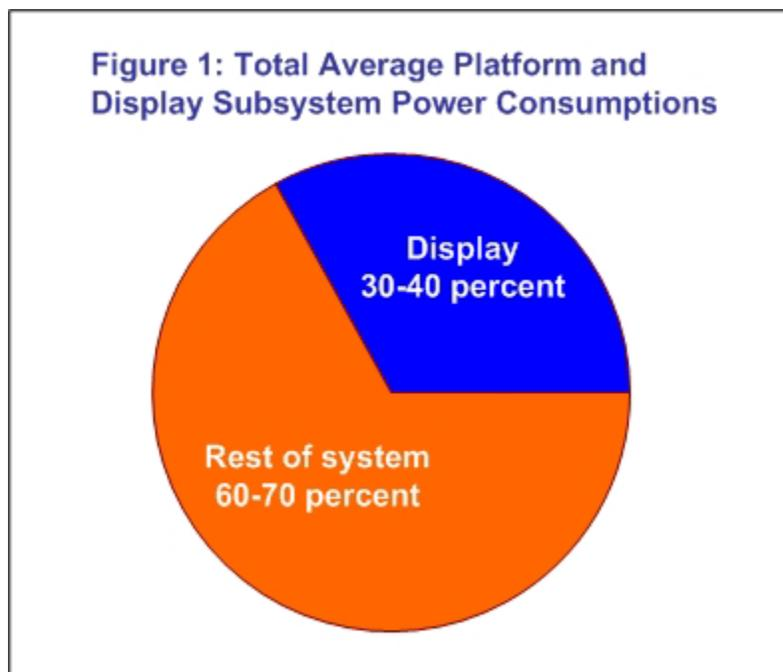
The total display subsystem power consumption includes power consumed by the display panel electronics, as well as the display panel backlight system, including the backlight inverter module.
